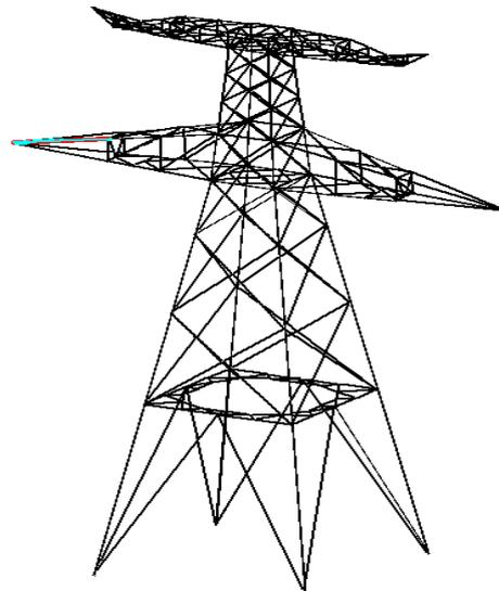
**Fig 4.1.1. Danube configuration of tower**
