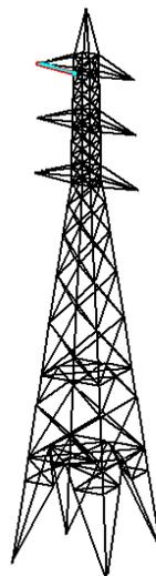
**Fig 4.11.2 Vertical configuration of a double circuit tower**
