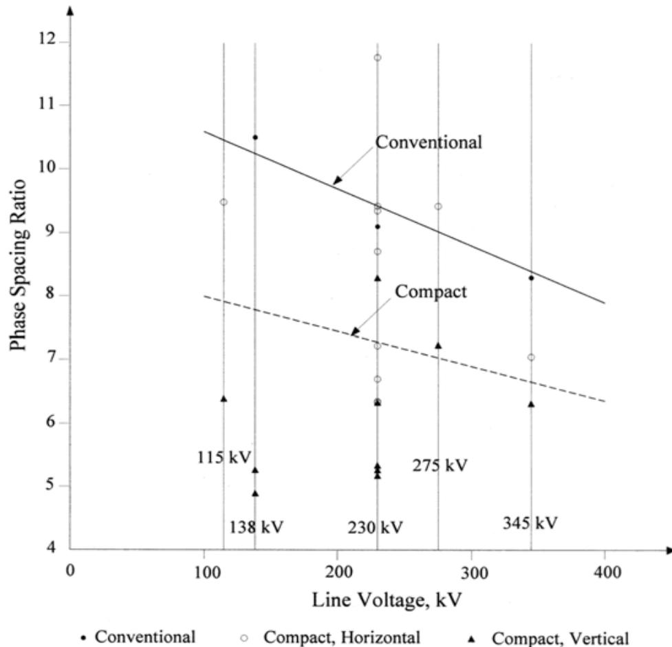
Figure 2.1.4:  $d_{pp} / d_{98\%}$ , for Traditional and Compact Transmission Lines
