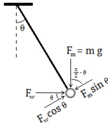
Figure 2.1.5: Blowout Pendulum Model
