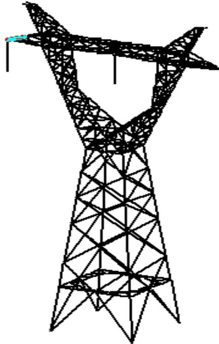
**Fig 4.1.1.3 Horizontal configuration of a single circuit tower**
