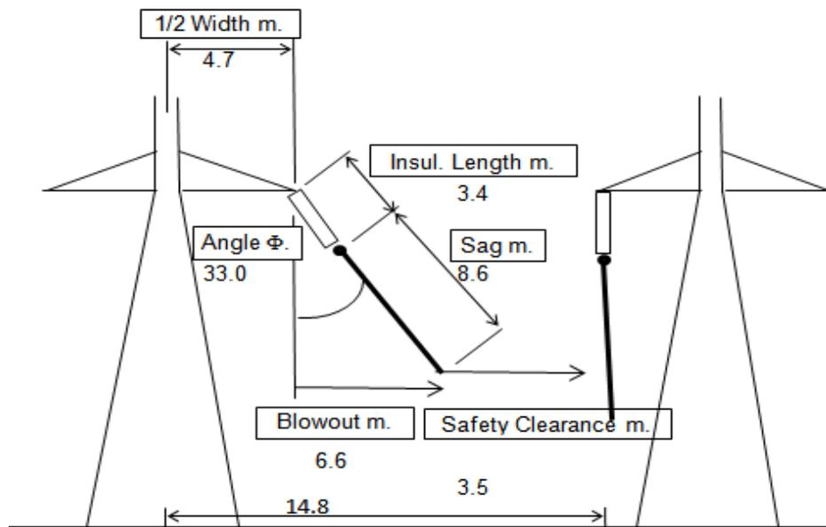
Fig 4.1.3 Illustration calculation of required way leave
